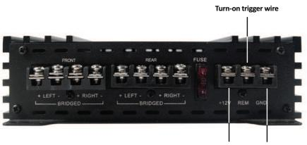
+12 volt at Battery positive terminal Ground to chassis
