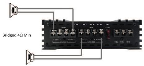
High power stereo using dual mono bridge hookups requires that the speakers be a minimun of 4 Ohms impedance each.
