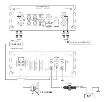
High-level input wiring
