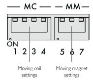
Set the switches up (OFF) or down (ON) according to the following tables.
