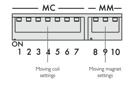
Set the switches up (OFF) or down (ON) according to the following tables.
