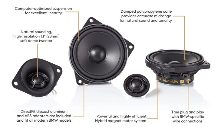
The 2-way IP-BMW42 component system was designed for music lovers wanting to upgrade their original BMW speaker system with a dynamic, Hi-Fidelity sound. Featuring DirectFit, the unique 4-inch (100mm) chassis design with supplied mounting brackets, easy snap-in 28mm tweeters, and factory wire connections allow the IP-BMW42 to fit modern BMW models without the need for modification.
