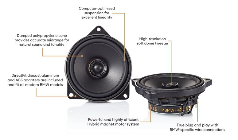
The IP-BMW4C coaxial system was designed for music lovers wanting to upgrade their original BMW speaker system with a dynamic, Hi-Fidelity sound. Featuring DirectFit, the unique 4-inch (100mm) chassis design with supplied mounting brackets and factory wire connections allow the IP-BMW4C to fit modern BMW models without the need for modification.
