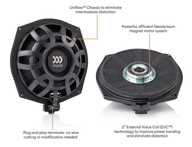
The IP-BMWSUB82 subwoofers are the ideal way to improve the bass in your BMW. The ultra slim 8-inch (200mm) subwoofer delivers accurate, powerful bass thanks to Morel's innovative EVC™ motor topology with a powerful neodymium magnet and large 2-inch voice coil. Using our DirectFit design, the BMW-specific chassis and plug-and-play connectors make for quick and easy installation into all BMW models with under-seat subwoofers.
